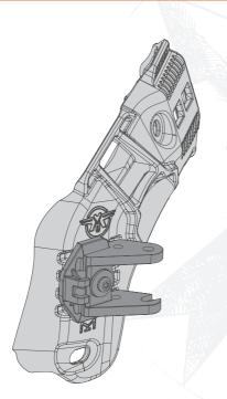
6 Reinstall center screw. Torque 16-18 in-lb. When properly tightened, AMP™ Helmet Adapter Arm assembly will funtion as it would on Ops-Core™ ARC™ Rail.
